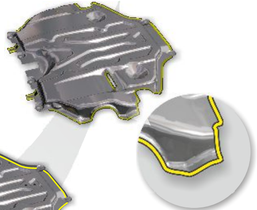
Restricken part with the desired part boundary and trim line after final AutoForm-Trim iteration
