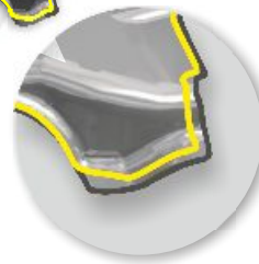
Restricken part with the desired part boundary and trim line after final AutoForm-Trim iteration
