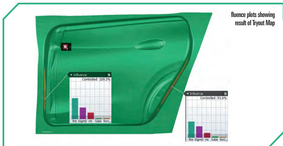
Robustness uses noise variables in the process that realistically cannot be controlled. SPI, based on AutoForm-Sigma<sup>plus</sup> (Systematic Process Improvement), is also used at Nissan to systematically evaluate the influence of design parameters on the robustness. SPI uses design variables which can be adjusted. To improve the draw process, SPI is used to create a Tryout Map which can then be used in conjunction with robustness.
