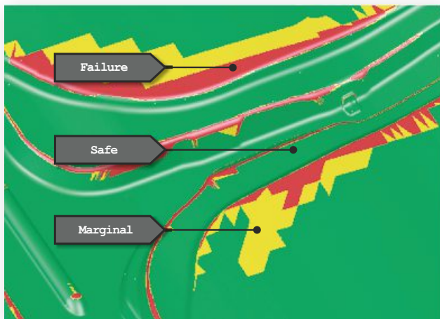
Tool failure (marked in red) by applying hard chrome plating
