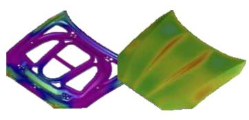
New Target for Hood Inner after Compensation
