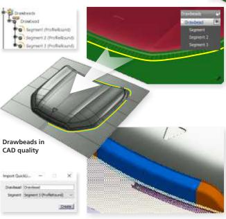
With AutoForm-QuickLinkforCATIA, drawbead parameters can be imported into AutoForm-ProcessDesignerforCATIA to efficiently support drawbead generation in CAD.
