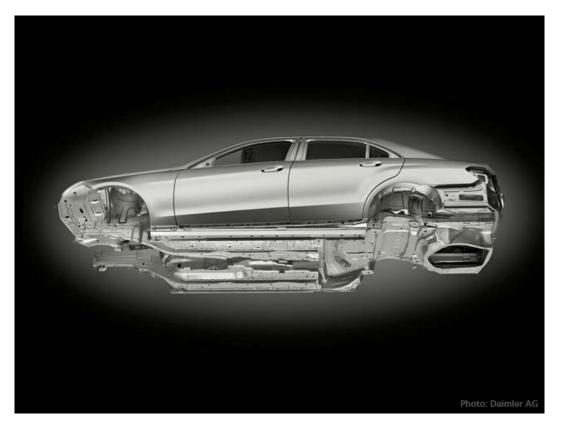
The amount of high-strength and ultra-high-strength steels used in the manufacturing of the new Mercedes-Benz E-class puts it in the lead.
