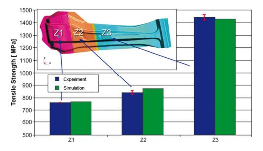
A comparison of measurement with simulation results demonstrates that AutoForm-ThermoSolver accurately calculates tensile strength.
