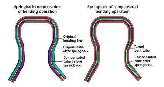
Springback compensation of bending operation
