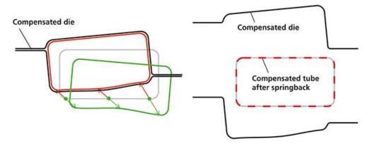
Springback compensation of hydroforming operation
