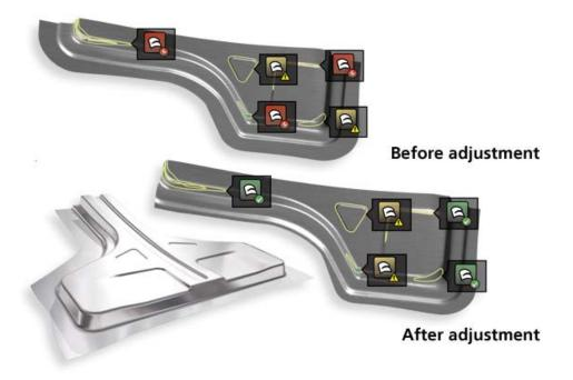
Issue identification: After adjusting stamping process parameters and running a new simulation, the issues indicate whether the forming behavior of a critical area has improved.
