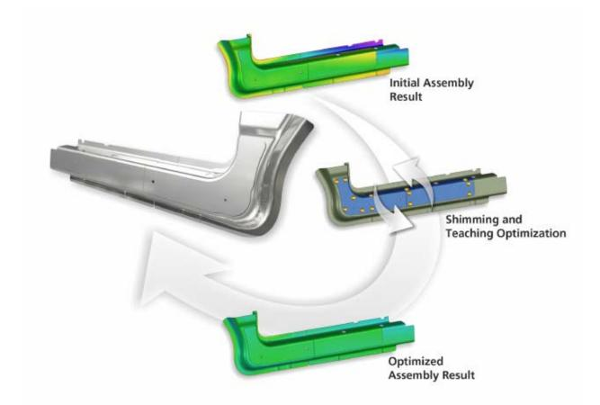
AutoForm Assembly R10 allows for assembly process optimization, providing users critical shimming and teaching strategies.
