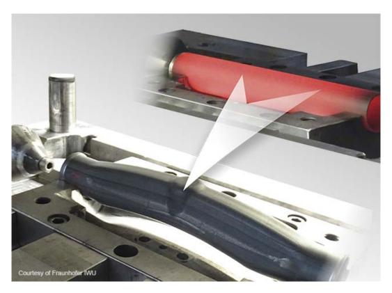
AutoForm TubeXpert enables users to simulate hot tube forming processes, including die face design, temperature and pressure control, applying advanced friction, systematic process improvement, and process robustness.
