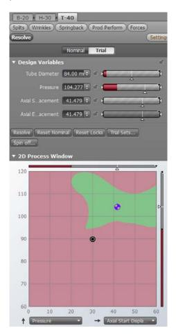
2D process window showing process formability depending on pressure level and movement of axial tools
