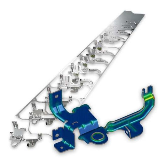
AutoForm software enables users to simulate the entire progressive die stamping process.
