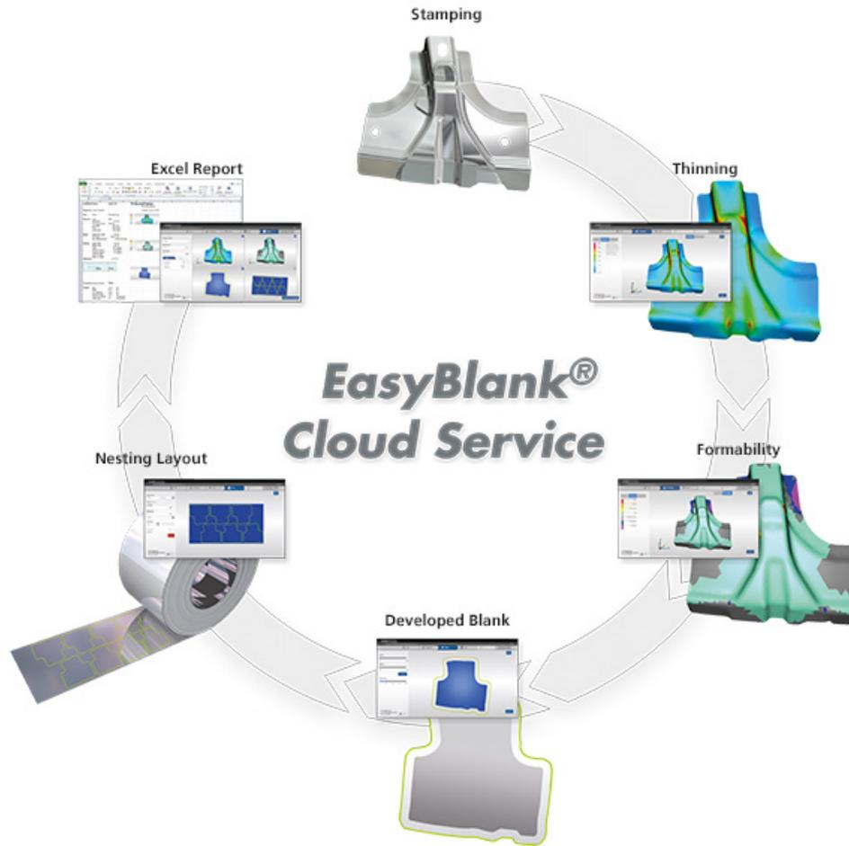
EasyBlank Cloud Service allows for the rapid determination of blank shape, early feasibility assessment and material cost estimation.
