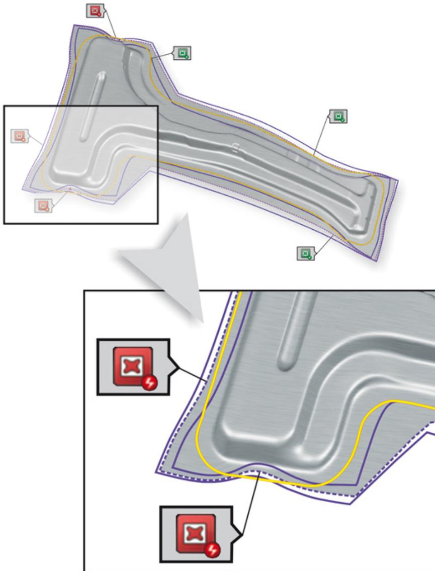
Draw-in is an added issue type which is suitable for semi-automatic results evaluation; the user can define draw-in target boundary as well as track the draw-in location and its progression by different available colors and icons.
