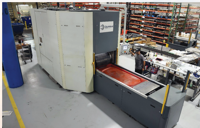
One of three high-pressure fluid-forming presses at Pimco. They employ tools produced following rigorous simulation to manufacture a variety of components for Piper aircraft.
