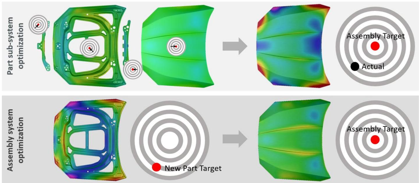
Figure 5: System optimization cuts over-engineering and waste
