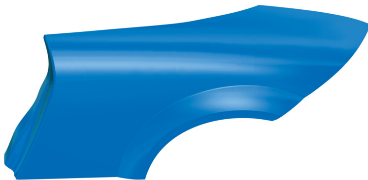
Figure 2-A: The part geometry (CAD surfaces) of an Audi TT rear fender.
