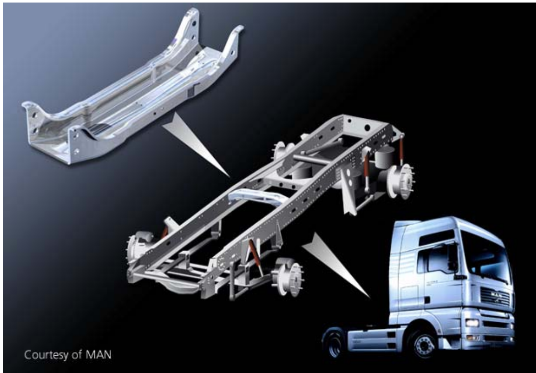
Cross member of semitrailer tractor frame (TGA)
