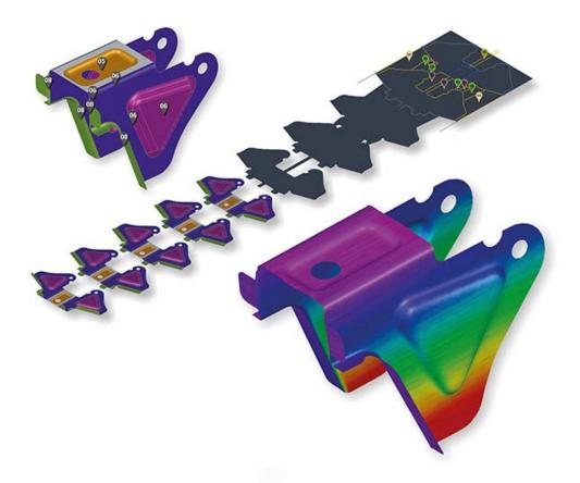
Blank plan and bend plan: AutoForm<sup>plus</sup> R7 new functionalities enable users to efficiently plan and simulate (e.g. springback) progressive dies.
