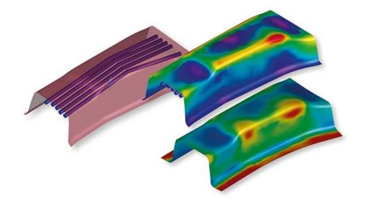
Cooling channels – tool design, tool temperature and sheet temperature.
