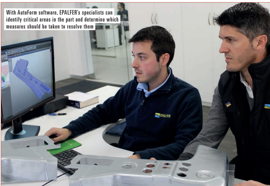
Above: AutoForm software enables EPALFER to select the process parameters and tool geometry for robust stamping processes
